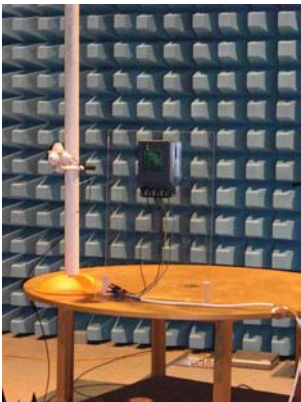
61000-4-3 RFI 30V, frontal, vertical polarity
