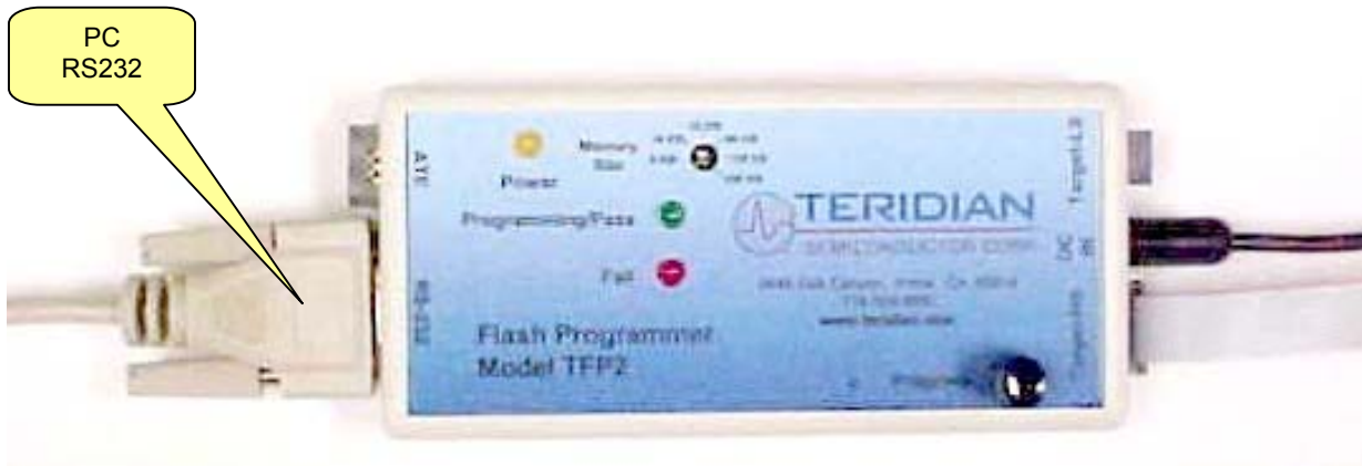
Figure 2-2: TFP2 RS232 Connection to PC
